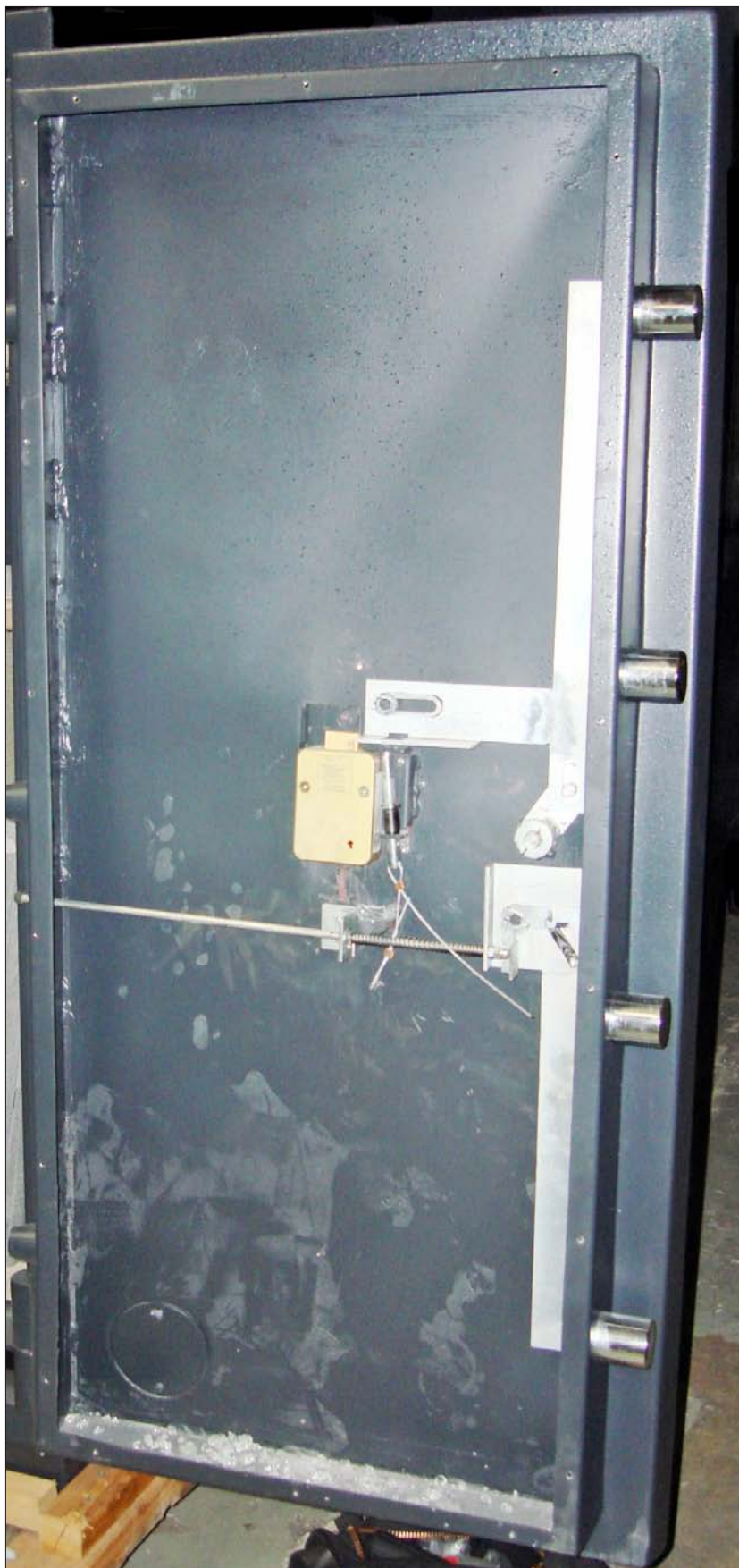
Back panel removed. This is a 1-way boltwork, with four door bolts on the opening side.
