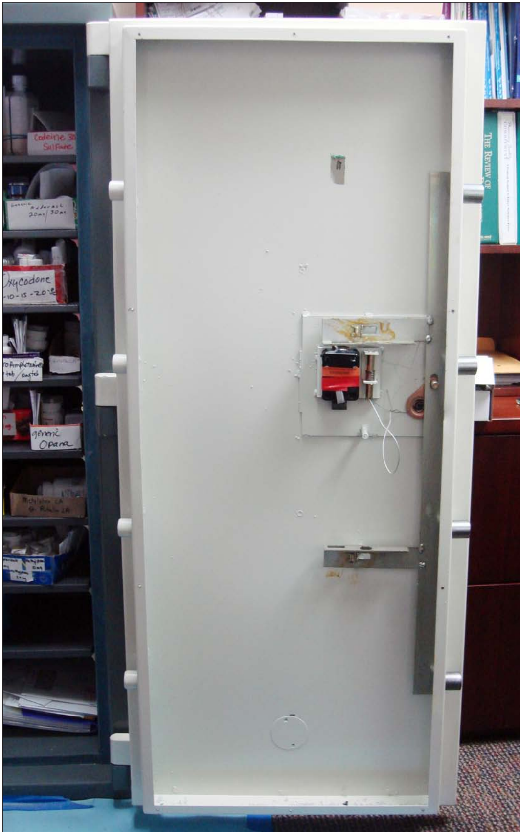
Back panel removed. This is a 1-way boltwork, with four door bolts, all on the opening side.
